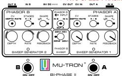
For a different program, one that utilizes GEN 2 to modulate PHASOR B, try setting the controls like template. Connect your instrument to the [PHASOR A INPUT] jack and the [PHASOR B OUTPUT] jack to your amplifier. Using this setting you can switch PHASOR A and PHASOR B on or off to create a phased signal with two different modulation types layered, or with the audio processed by a single phase section
