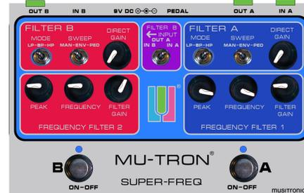
For surgical crossover and equalization applications. Set FILTER A to split upper-mid and high frequencies to one amplifier and set FILTER B to split low frequencies to another amplifier. Connect your instrument to the [FILTER A INPUT] jack and the [FILTER B OUTPUT] jack to your amplifier. Set FILTER A to act as a BAND PASS or HIGH PASS filter. Set FILTER B to act as a LOW PASS filter. This is a very useful combination to EQ and route "dry" and "wet" signals, such as in an effects chain.
