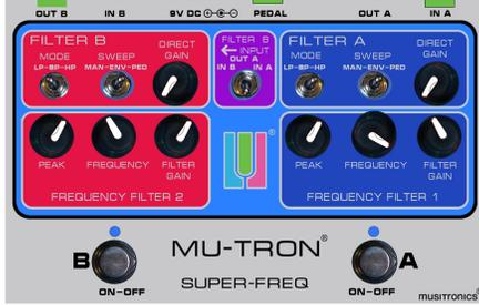
Connect a recommended power supply to the power socket at the rear of the SUPER-FREQ. Connect expression pedal to pedal jack using TRS 1/8 to 1/4 adaptor. Connect your instrument to the [FILTER A INPUT] socket at the rear of the pedal. Connect the [FILTER B OUTPUT] to your amplifier. Using the visual guide below, set the controls to the above template. Make sure both channels are turned on – both channel LEDs should be lit – then play something and turn up your amp.
