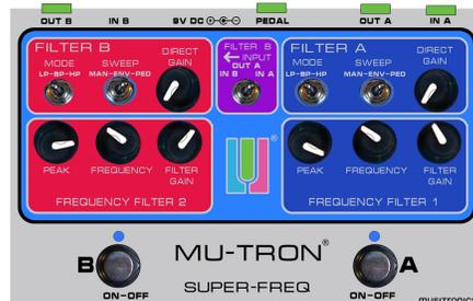
Connect your instrument to [FILTER A INPUT] on the rear of the pedal, your primary amplifier to [FILTER B OUTPUT], your secondary amplifier to [FILTER A OUTPUT], then set the controls like template. There is a noticeable 'movement' of the input audio signal between the two amplifiers. Try to experiment with various LOW PASS, BAND PASS, and HIGH PASS settings on either side. By actuating different frequency ranges simultaneously, you can achieve some weird COMB-FILTERING effects.
